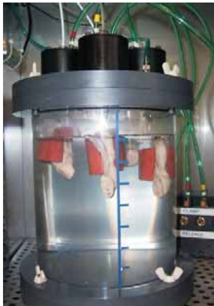
Pressure tank with Intran & Koala catheters covered with pig uteri and latex tubing obstruction.
